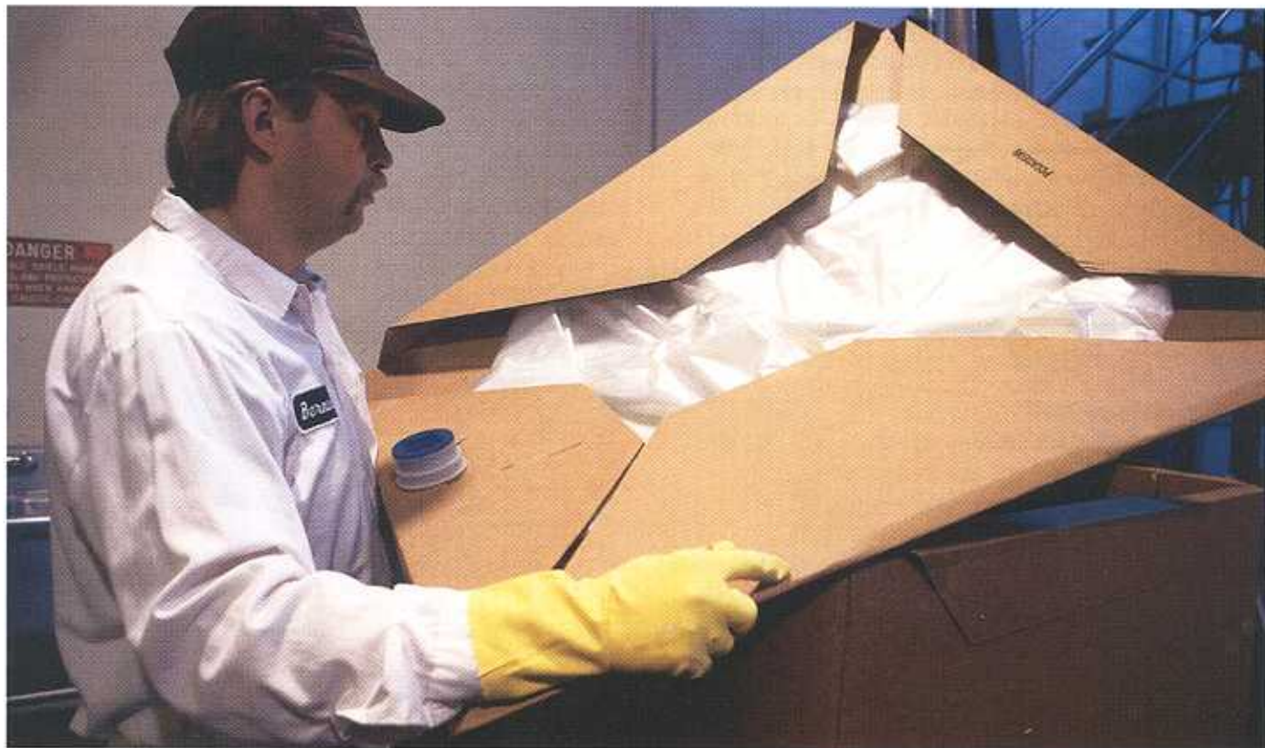
The bag liner is supplied in a corrugated cassette that can be easily inserted into the outer corrugated sleeve.
