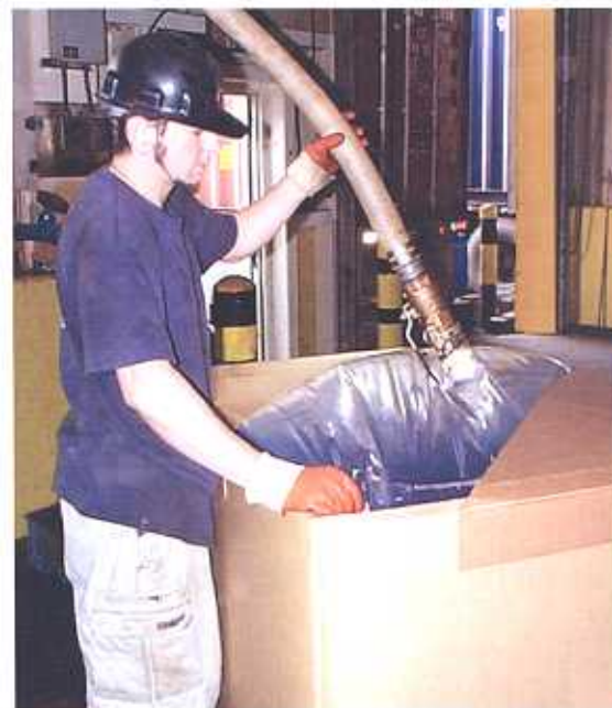
Today, one operator is required to fill an IBC, using a filler that allows the operator to start setting up the next IBC while this one is filling.
